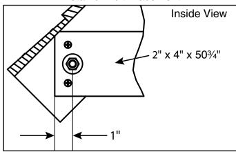
Predrill -1/8" dia. for #8 x 21/2" deck screws 3/8" dia. for 3/8" x 31/2" hex bolts
