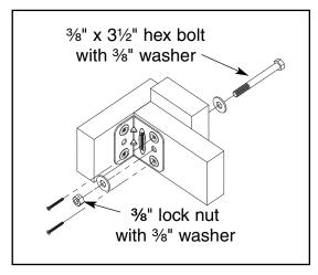
Securing through two boards use 3/8" x 31/2" hex bolt.
