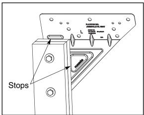
Rear View of bracket and post assembly showing correct position.
